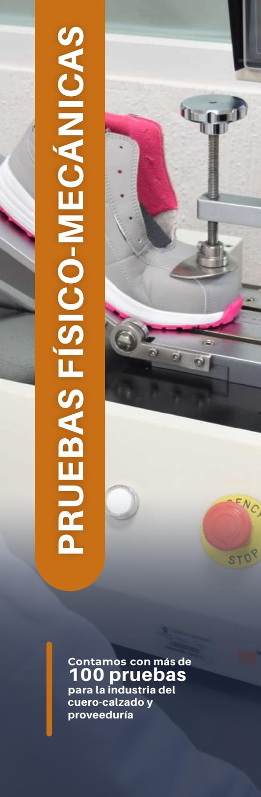
A white and pink sneaker is positioned on a mechanical testing machine. The machine has a vertical rod with a circular weight on top, which is about to impact the shoe. The shoe is held in place by a metal fixture. The machine is white and has a red emergency stop button with a yellow label that says 'EMERGENCY STOP'.
